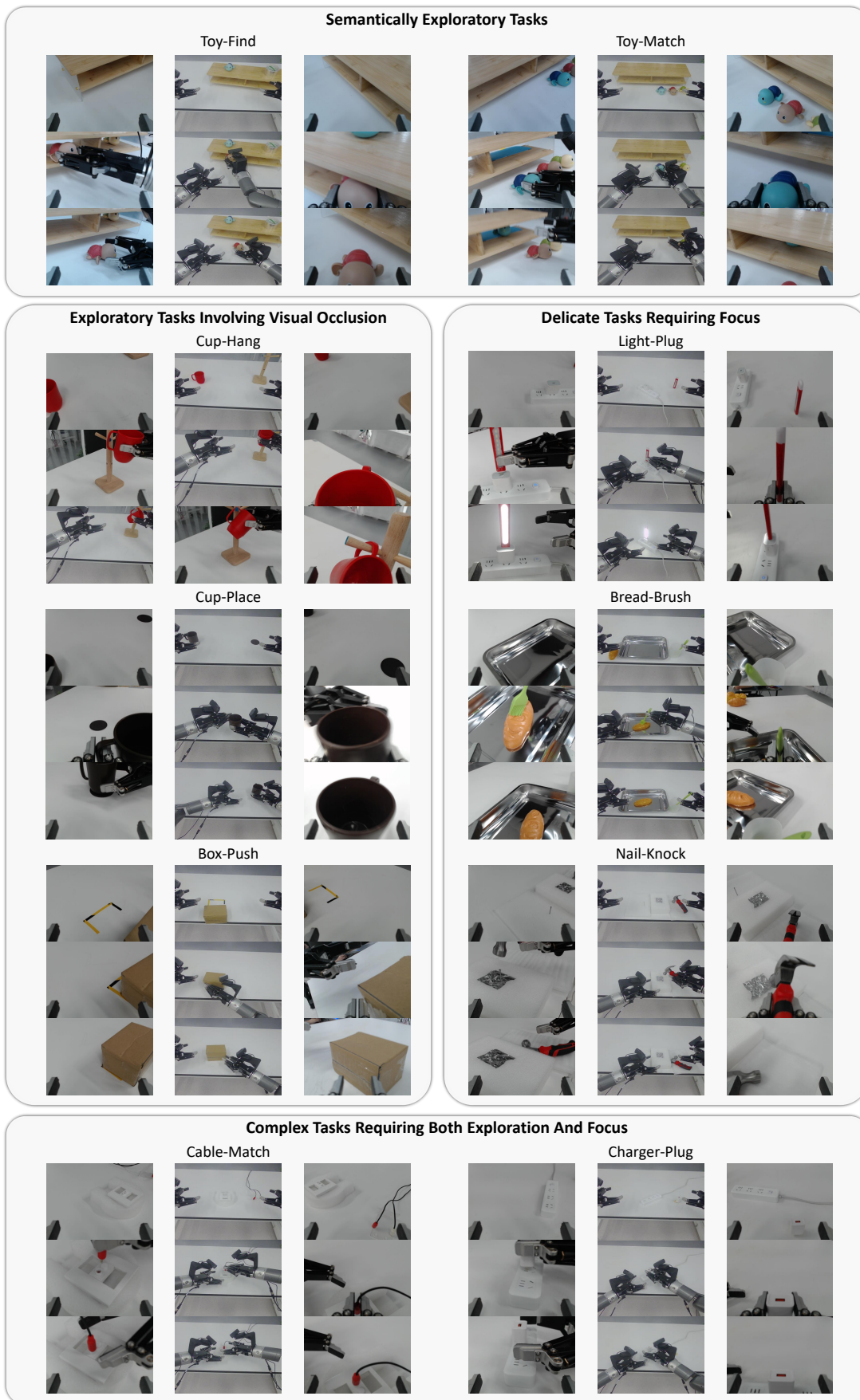
Fig. 1: An illustration of the BAPData dataset collected for the 10 tasks in EFM-10. The left wrist-view images (left column), main-view images (middle column), and right wrist-view images (right column) are shown temporally for each example.
